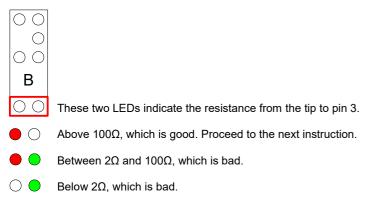
The problem is due to a short circuit between the contact spring and the inside of the barrel when the tip is pressed. Remove the tip and inspect the contact spring for breaks, contamination or de-lamination of the wire.
